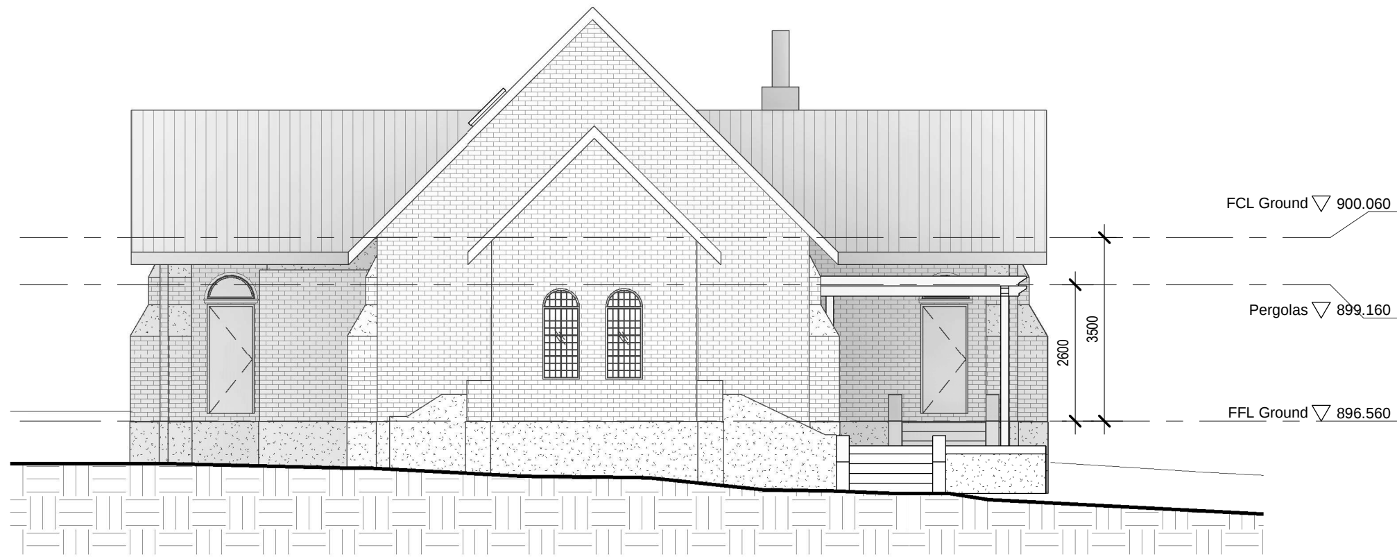
1 DA101 ELEVATION 1 : 100 EAST ELEVATION
